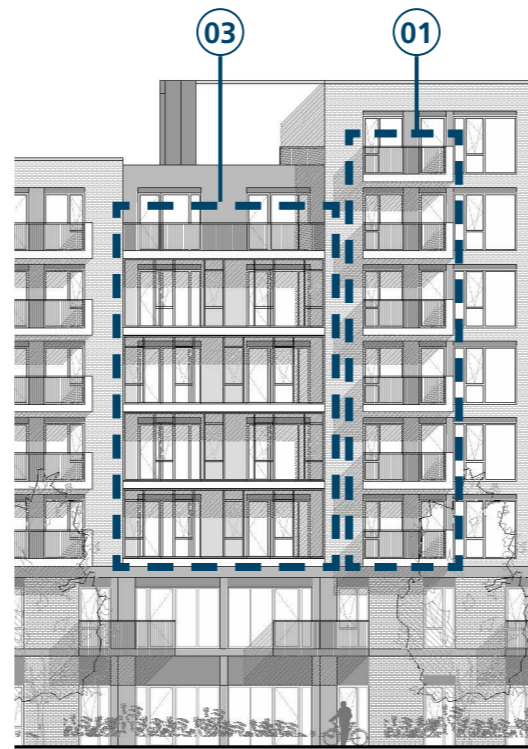
03 01 ▲ Typical section of facade with both projecting balconies stacked in columns and recessed balconies acting as a break between different building volumes
