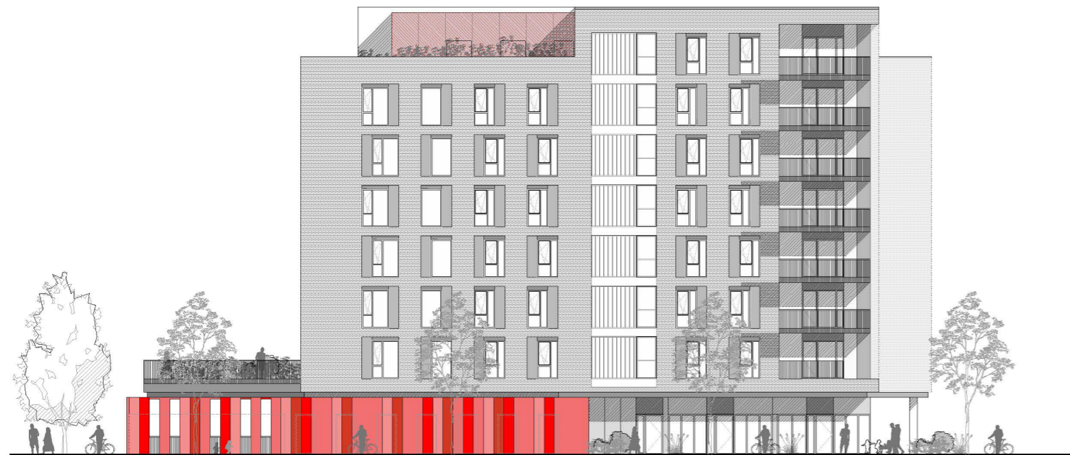
▲ Red material cladding facade at ground levels resulting in an external screen housing the creche outdoor play spaces
