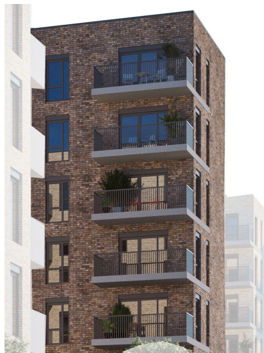
▲ CGI View of typical corner balconies with concrete string detail on return elevation
